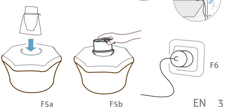
4. Plug the outdoor power transformer (9) into a water safe outlet [F6]. Use the extension cord to set the trap at distances up to 33 ft from the power transformer. When the power is turned on, the shutter will automatically tilt open.
